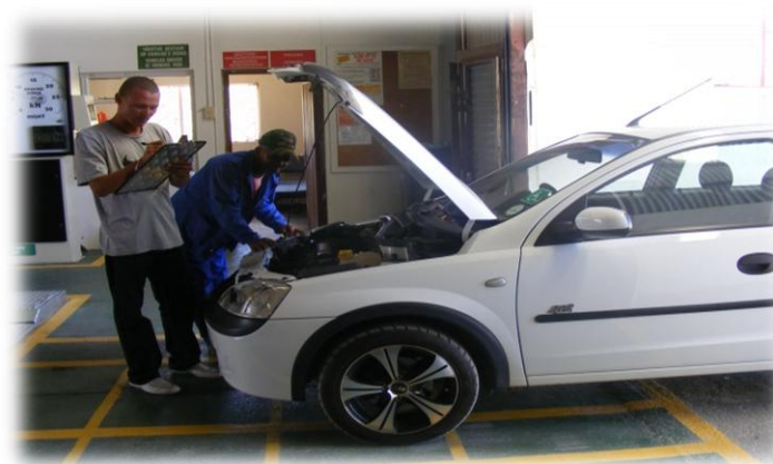
Examiner of vehicles busy with a roadworthy test of a light motor vehicle
